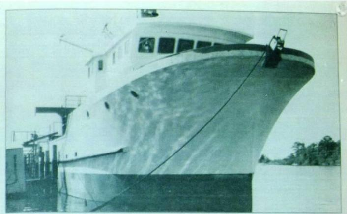
Yale built 100' hull over hulls built from fiberglass, but Master Marine is the only U.S. builder to have constructed a 100' fiberglass vessel. The company plans to build even larger vessels of 110' and 120'.
