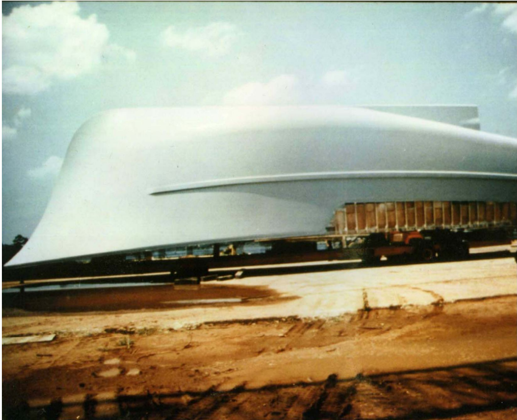
Hull plug for the "One Ocean I" (85 ft, Mississippi shipyard)
